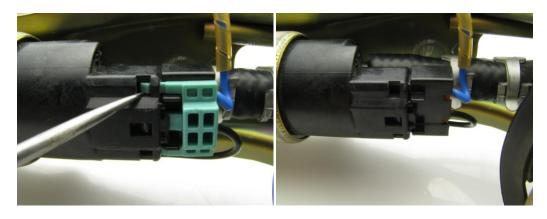
2 – disconnect the electrical connector and remove the fuel sock
