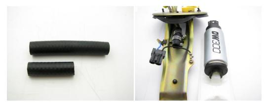
5 – install the supplied fuel sock on the DW200/300 with the fuel sock retainer and install the pump into the assembly
