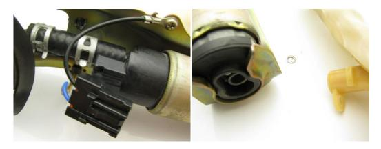
3 - remove the OE pump from the assembly, do not discard the OE pump isolator
