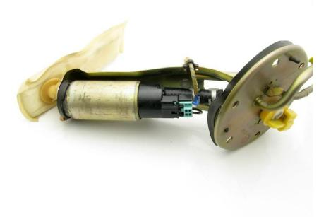
1 – remove the green retainer from the electrical connector, it may be discarded if damaged during removal
