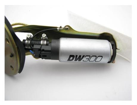
7 – reinstall the assembly into the fuel tank and attach a length of hose to the outlet of the pump assembly allowing it to drain into a fuel safe container and prime the fuel pump assembly
